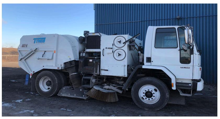
In early 2020 Stelco purchased a Tymco Regenerative Sweeper Truck for yearround road dust control. The vacuum action of this unit requires no water, allowing for use in freezing temperatures that traditional sweepers cannot operate in.
